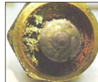
Polymerizing sealants remain liquid until exposed to moisture or oxygen
