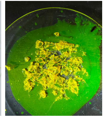
Polymerizing sealants remain liquid until exposed to moisture or oxygen
